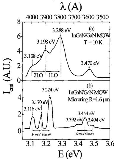
FIG. 3. Low-temperature (10 K) optical emission spectrum from (a) an InGaN/GaN MQW sample prior to microring fabrication; (b) an InGaN/GaN MQW microring with an outer diameter of  $3.2 \mu\text{m}$  and a ring width of about  $0.7 \mu\text{m}$ . Optical resonance modes of the WG-mode type are observed in the microring in (b).
