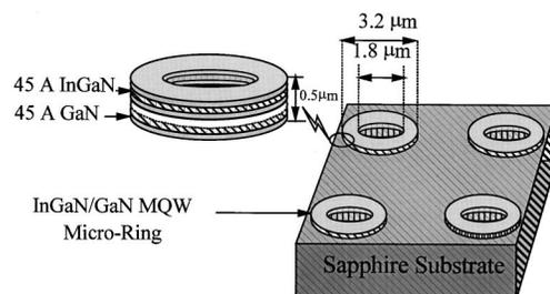
FIG. 1. Schematic diagram of representative InGaN/GaN MQW microring fabricated by photolithography patterning and dry etching.
