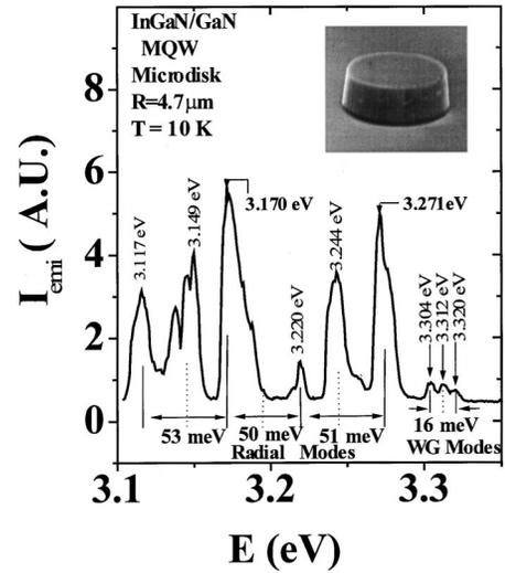
FIG. 4. Optical emission spectrum of an InGaN/GaN MQW microdisk with a diameter of  $9.4 \mu\text{m}$ . Both the WG and radial modes are observed in the microdisks.
