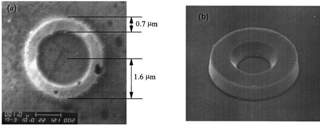
FIG. 2. Scanning electron microscopy (SEM) images of an InGaN/GaN MQW microring fabricated by (a) ion-beam etching and (b) inductively coupled plasma (ICP) etching. Ion-beam etching-induced damage are observable in the cap layer of the ring in (a).
